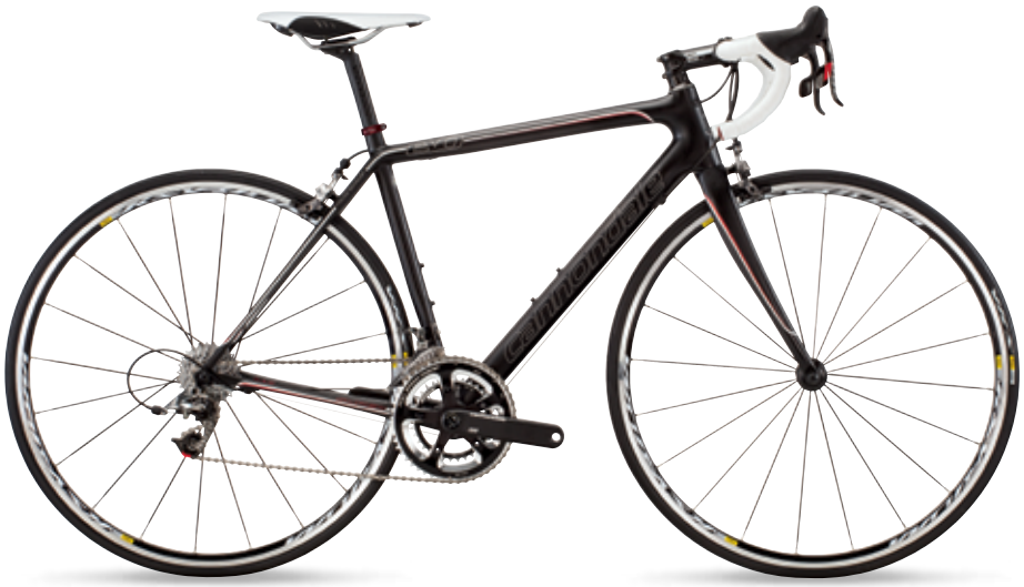
SUPERSIX EVO WOMEN'S 2 RED FRAMESET: SuperSix EVO Women's, BallisTec Carbon WHEELSET: Mavic Ksyrium Equipe S WTS CRANKSET: HollowGram Si, 50/34 COCKPIT: Cannondale C1/C2 Women's GROUP: SRAM RED 22 COLORS: Carbon w/ Ruby Red, Silver, Pearl - Matte (01)
