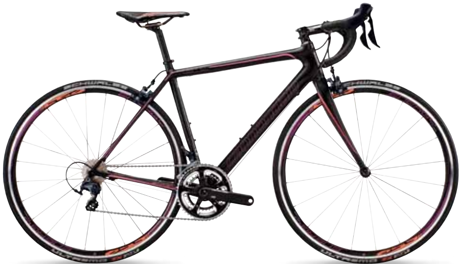
SUPERSIX EVO WOMEN'S 2 RED FRAMESET: SuperSix EVO Women's, BallisTec Carbon WHEELSET: Mavic Ksyrium Equipe S WTS CRANKSET: HollowGram Si, 50/34 COCKPIT: Cannondale C1/C2 Women's GROUP: SRAM RED 22 COLORS: Carbon w/ Ruby Red, Silver, Pearl - Matte (01)
