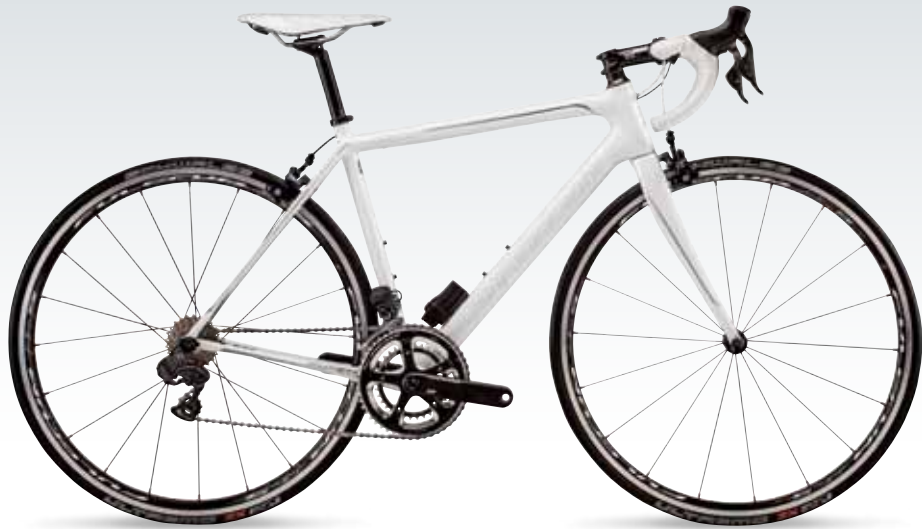
SUPERSIX EVO WOMEN'S ULTEGRA DI2 FRAMESET: SuperSix EVO Women's, BallisTec Carbon, Di2 WHEELSET: Fulcrum Racing 5 CRANKSET: HollowGram Si, 50/34 COCKPIT: Shimano Ultegra Di2 6870 GROUP: Cannondale C1 Women's COLORS: Magnesium White w/ Super Sparkle Silver, Pearl - Gloss (01)
